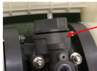
Tighten the replacement CAP A until the gap disappears.
