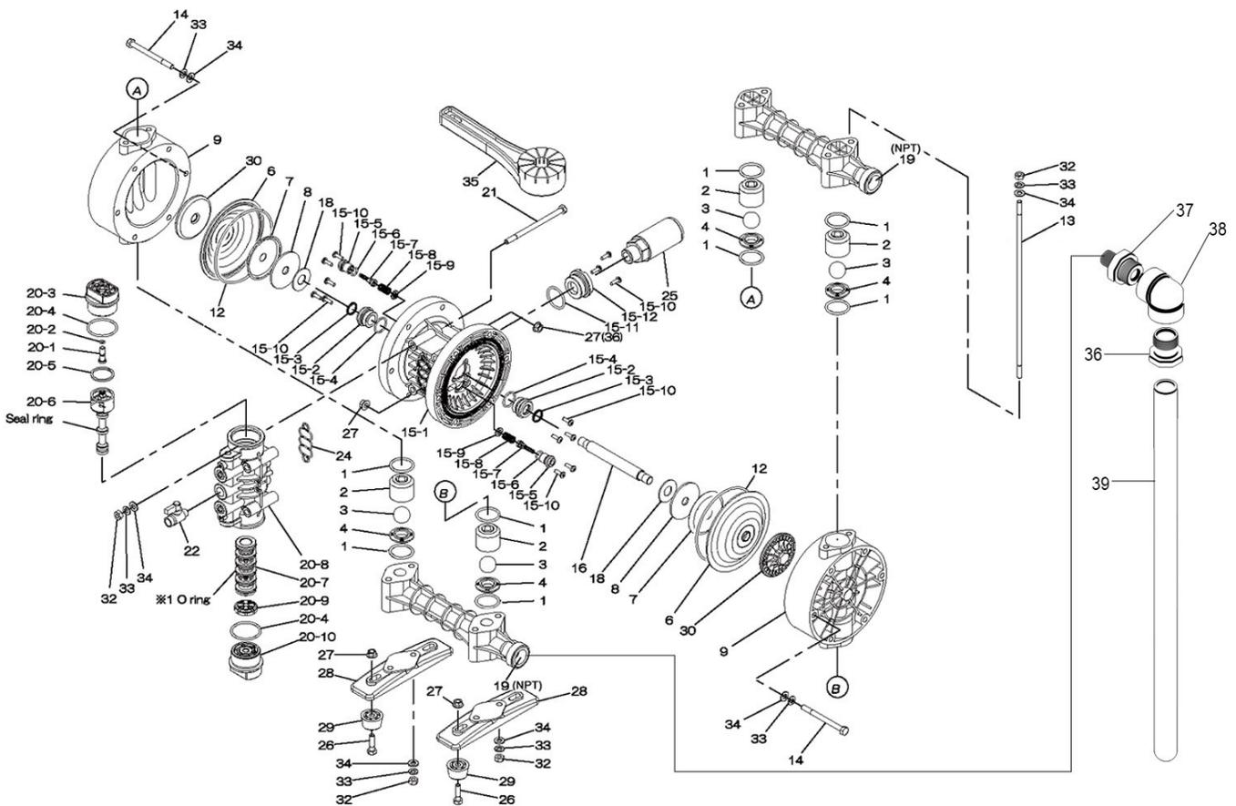
Air Operated Double Diaphragm Pump
