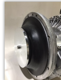
Slide on abrasion pad and center disk. Curve of center disk to face in.
