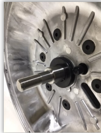
Insert cushion to center rod, where used.
