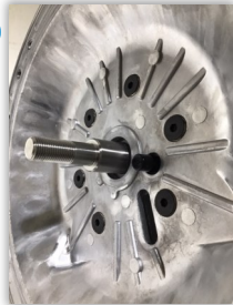
Insert center rod to center body.
