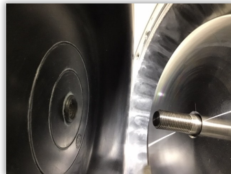
Slide on diaphragm onto center rod. Diaphragm lip sits flush against center disk.
